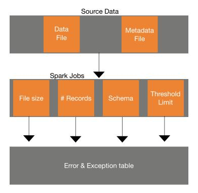
The source data includes different data files and their corresponding metadata files which consists of metadata such as file size, no. of records, schema etc. A series of spark jobs can be designed to run on the source files once the data is ingested in the HDFS. These jobs handle the error exceptions for different scenarios.
